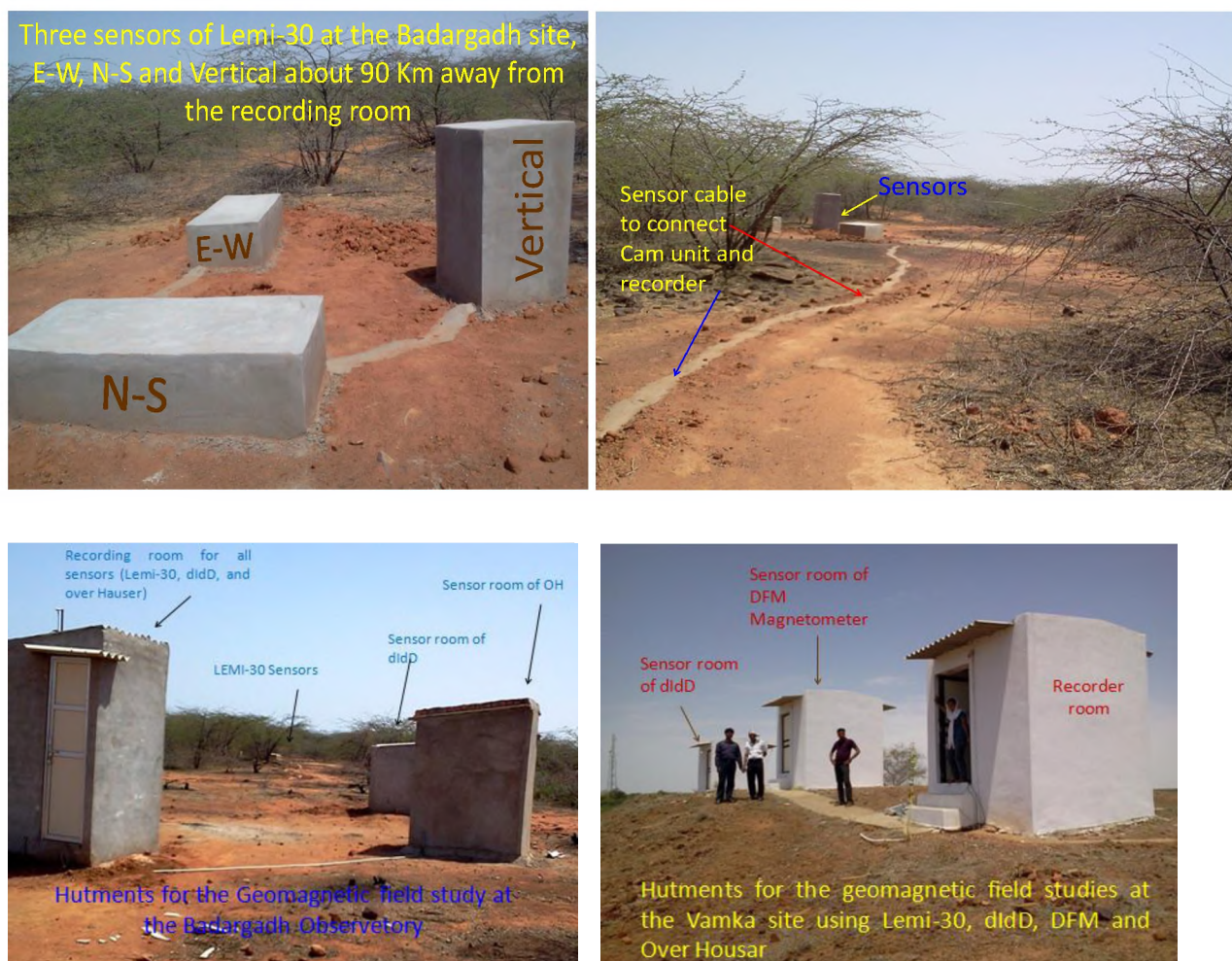
Fig.7.1 Specialised pits and non-magnetic huts for Magnetometers
