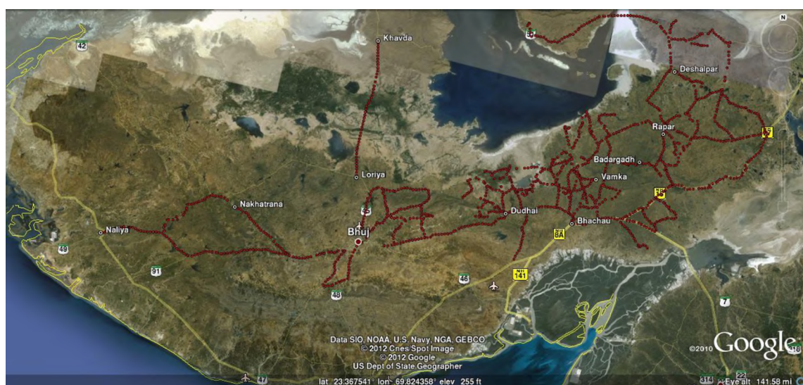
Fig. 3.2.1: Gravity lines covered by ISR at intervals of 1km or less. Gravity Stations have been located over permanent landmarks available in Survey of India, degree sheet No 41 I & 41 E
